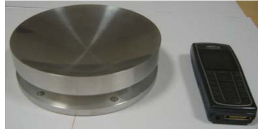
Fig.3. Cold cathode of gas-discharge EB gun BTP-450
