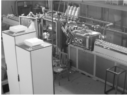
Fig.5. Gas-discharge EB guns BTP-100 at EB-PVD installation
