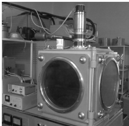
Fig.6. Gas-discharge EB gun BTP-60 at R&D installation
